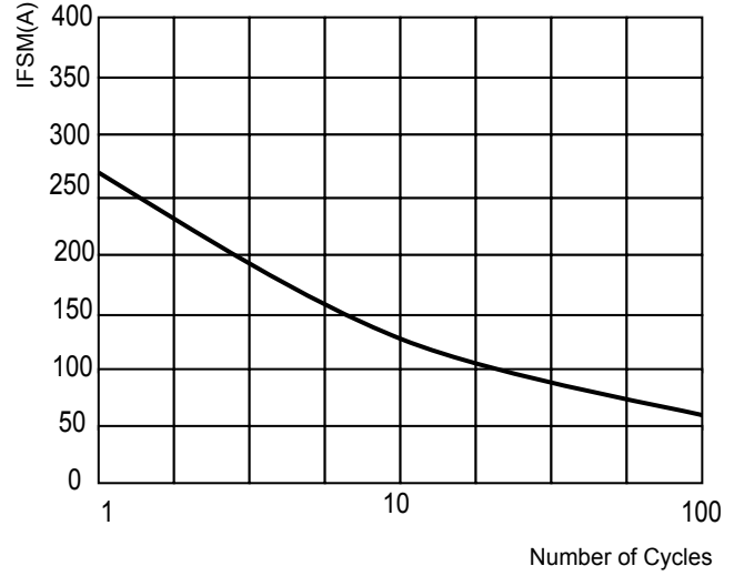
FIG.2-MAXIMUM NON-REPETITIVE SURGE CURRENT
